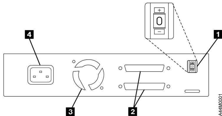
Figure 2. Rear View of the 7208 Model 345 Tape Drive
