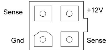
Figure 10. Power Supply Connector J2
