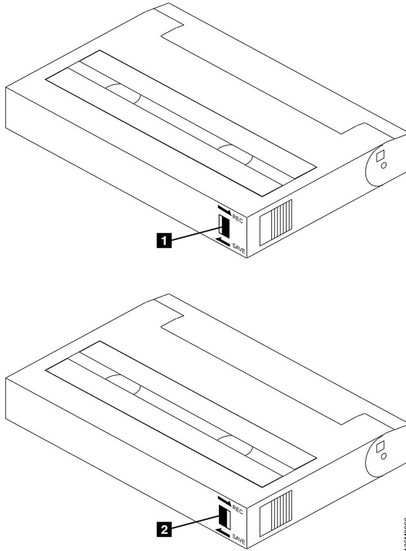
Figure 7. Setting the Write-Protect Switch
