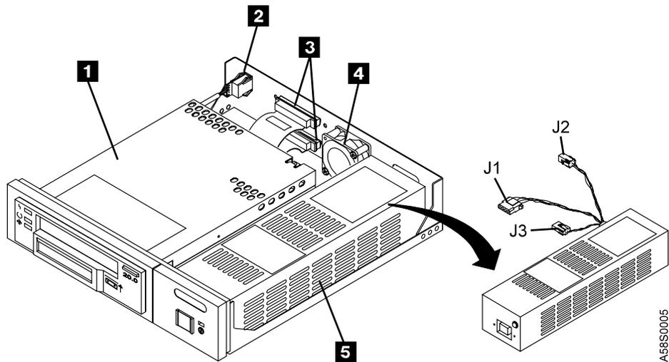
Figure 4. Internal View of the 7208 Model 345 Tape Drive
