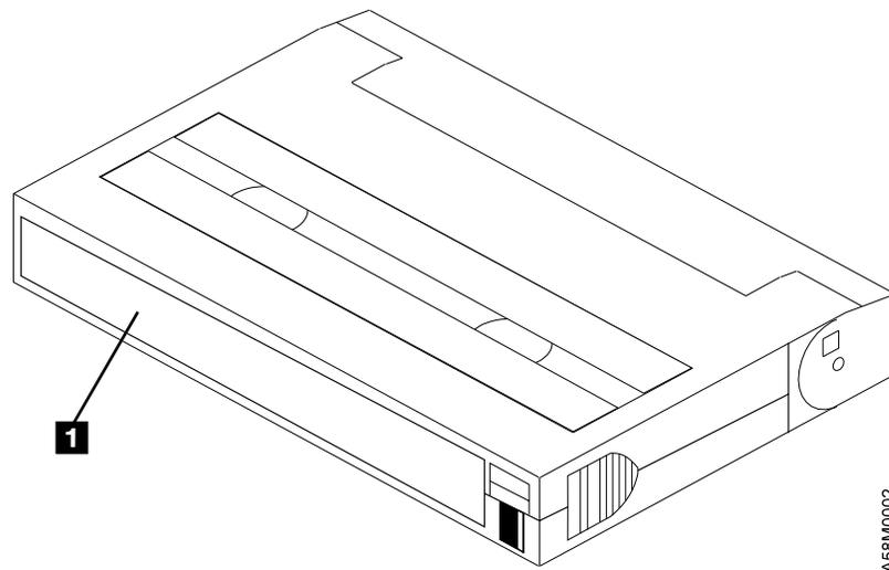
Figure 6. Placement of Label on an 8mm Data Cartridge
